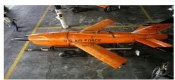
**Fonte:** <a href="http://olive-drab.com/idphoto/id\_photos\_uav\_bqm34firebee.php">http://olive-drab.com/idphoto/id\_photos\_uav\_bqm34firebee.php</a> <a href="http://olive-drab.com/idphoto/id\_photos\_uav\_bqm34firebee.php">Figura 04 - VANT Firebee</a>
